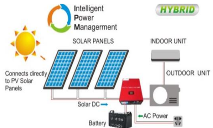
Figure 17: Hybrid Solar AC using DC & AC power
