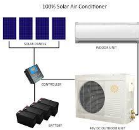
Figure 16: Solar AC off grid type
